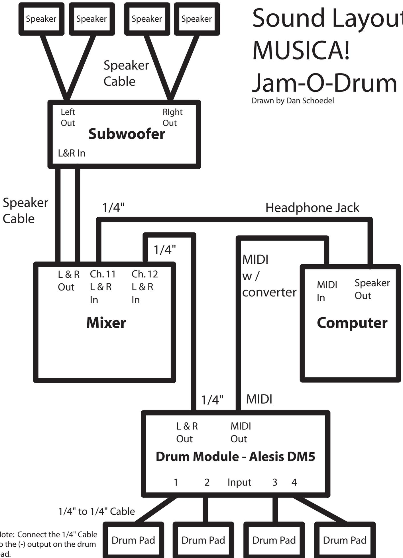
Note: Connect the 1/4" Cable to the (-) output on the drum pad.
